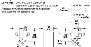
This adaptor permits the installation of a D03 valve on a D05 manifold. This adaptor, unlike \*D03D05VABA\*, properly orients the A & B ports on the manifold to the respective valve solenoids.
