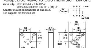
This adaptor permits the installation of a D03 valve on a D05 manifold. This adaptor, while low in cost, does not orient the A & B ports on the manifold to the respective valve solenoids.
